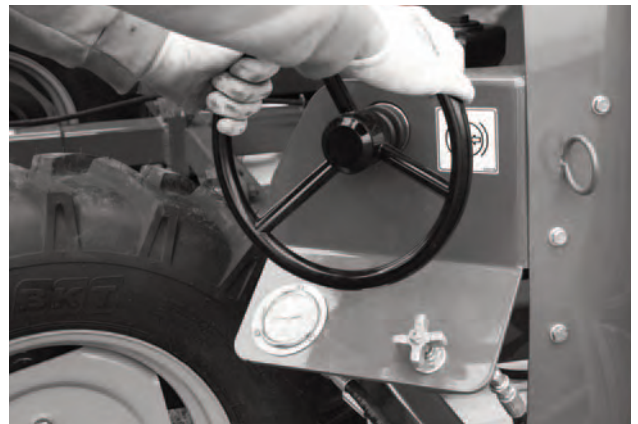
Figure 7 - Hydraulic brake system
