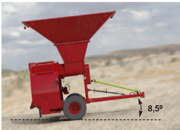
Figure 3 – Bagging machine parked against a slope
