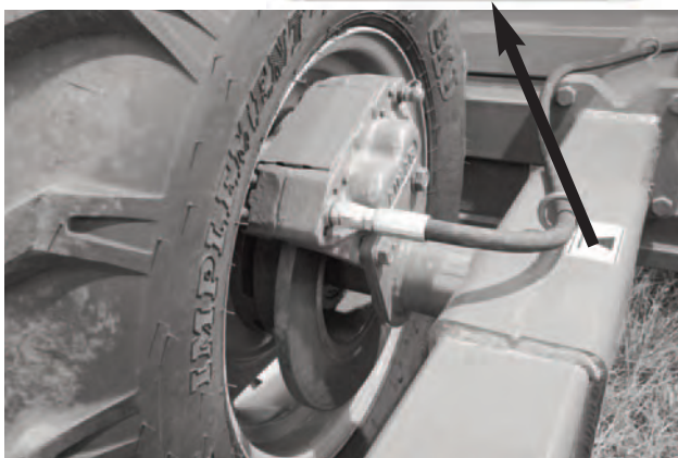
Figure 4 - Support point for jack location
