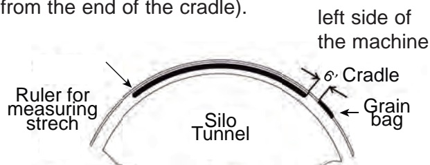
Figure 12- Positioning of the grain bag on the cradle
