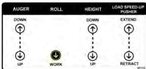
Figure 5.7 Switch valve lever into “ROLL” position.
