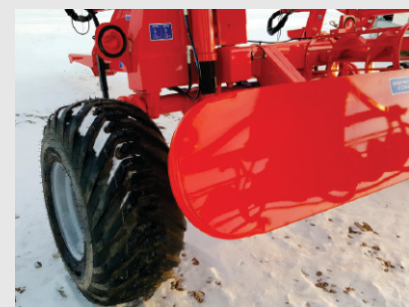
Grain pusher pan improves "end of bag" clean up & performance in tough grain conditions.
